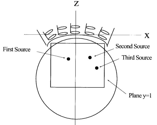
Fig. 1. Source and detector configuration assumed in computer simulation.
